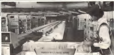
An automated bar-code sorter makes fast work of mail distribution in Washington, D.C.
